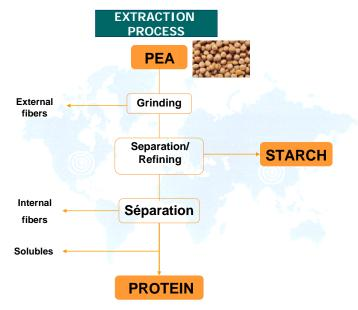
Fig. 2 : Pea extraction separation process
